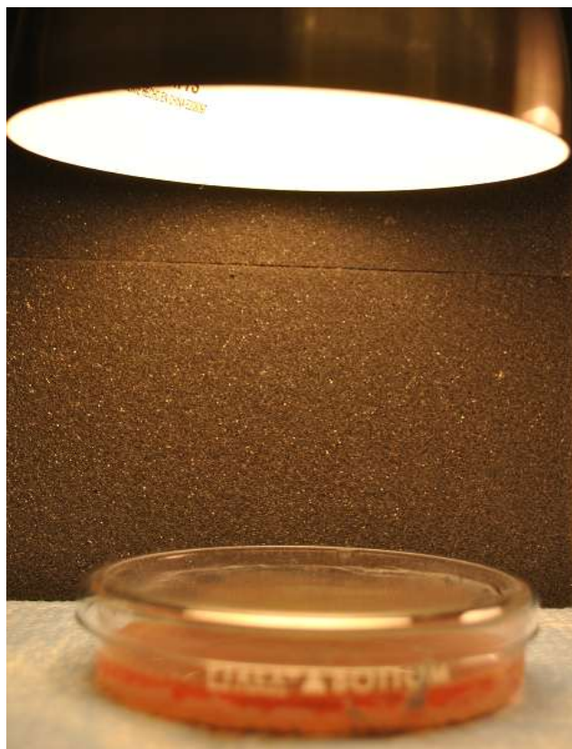
Figure 3.19: Setup for photodegradation of MO by G-TiO 2 under irradiation of 60 W normal bulb
