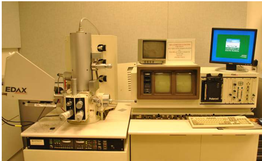
Figure 2.3: Scanning Electron Microscopy (SEM) and Energy Dispersive Spectroscopy (EDS) at USF
